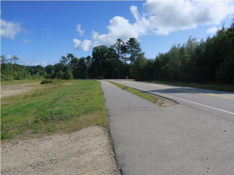
The site drops off from the elevation of the road. Ideally, the site would be raised for ease of access and more importantly, to raise higher above the flood plain.
